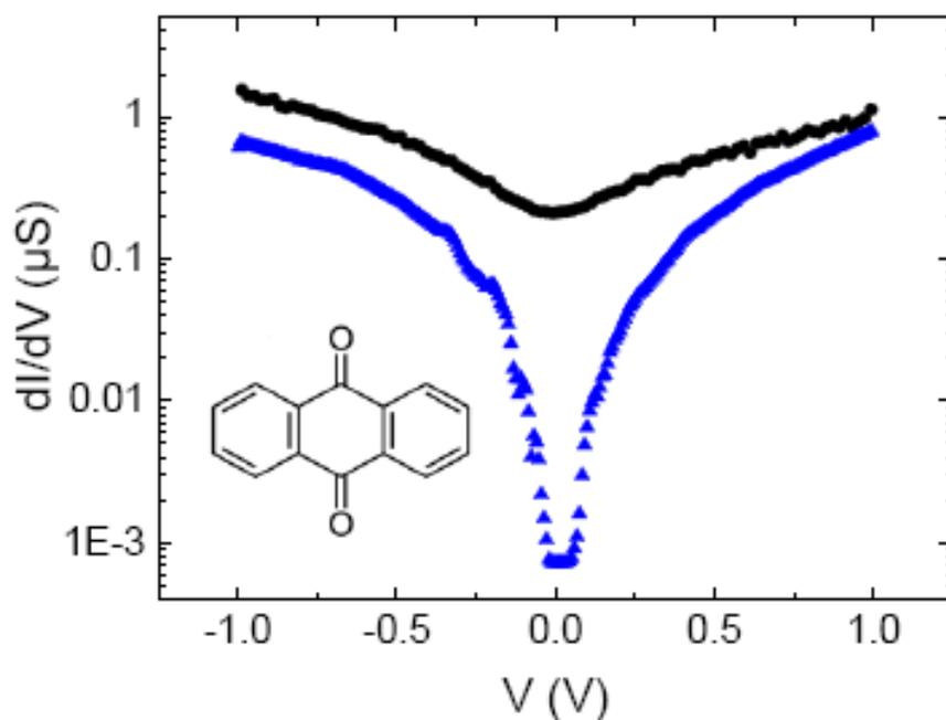
Figure 1. Measured  $dI/dV$  vs  $V$  data for an AQ-based junction at  $300\text{ K}$  (black circles) and  $4\text{ K}$  (blue triangles) with an area of  $30 \times 30\ \mu\text{m}^2$ . A pronounced antiresonance is present at low voltage.
